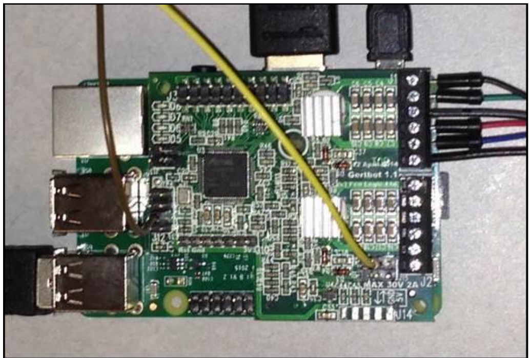
Fig.1b: Raspberry Pi 3 with mounted Gertbot. The yellow cable on the right connects to the open collector driver ODO, the brown cable on the left to +5V on the internal serial port.
