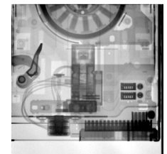
Neutron radiograph of a floppy disk taken by CAEP
