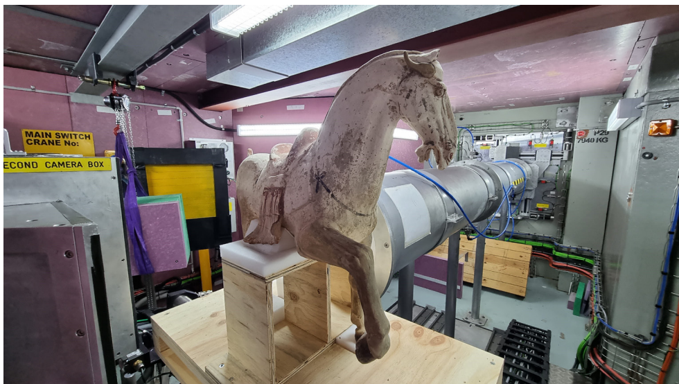
A T'ang Dynasty figure of a horse in position for neutron radiography.
