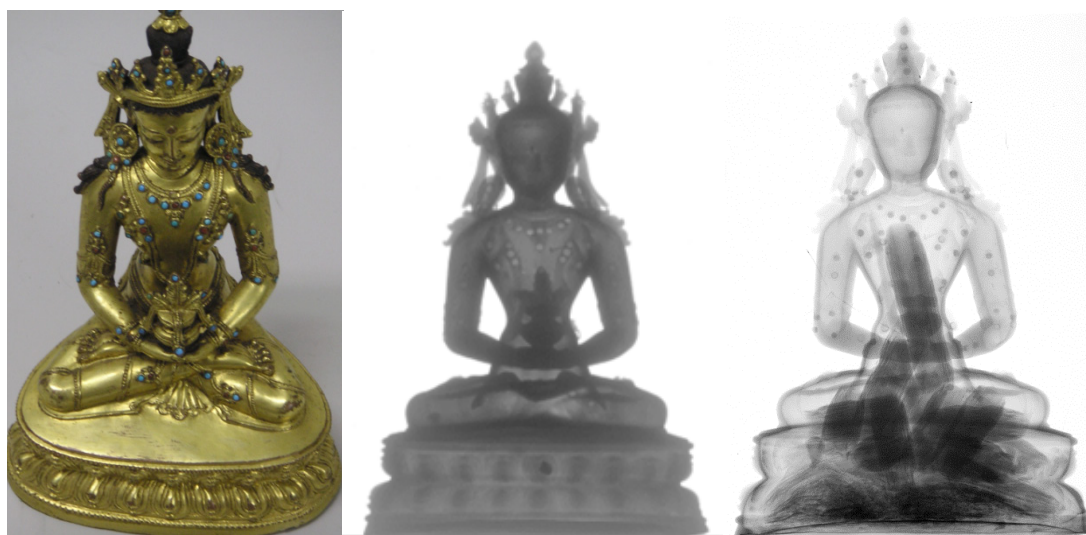
Fig. 1: Example of the study of an Buddhist bronze object: Buddha Amitayus, central Tibet, 17 th century; middle: X-ray image, right: neutron image
