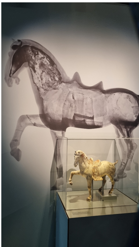
Neutron radiograph of the T'ang Dynasty horse, reproduced at full resolution at the entrance to the exhibition, revealing historical repairs made to the horse.
