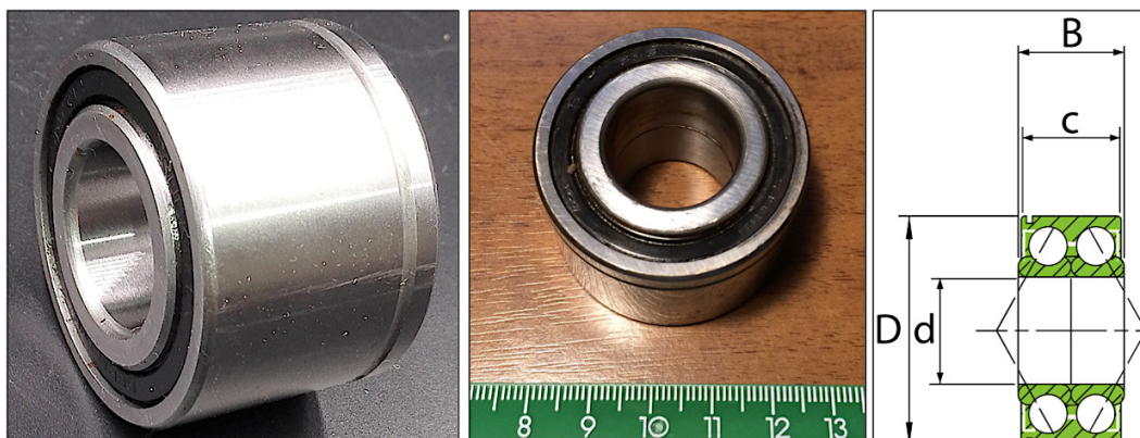
Fig. 1. The two investigated double-row DIN 100Cr6 bearings: new (left) and damaged due to the operation (centre); section (right). The indicated dimensions are: D = 42 ; d = 20 ; c = 29 ; C = 30 mm. The mass of each bearing is 178 g.
