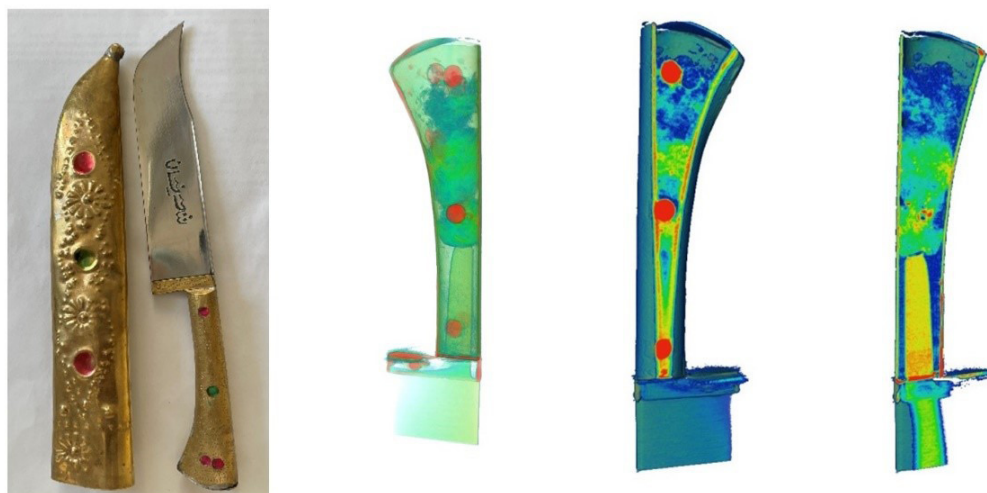
Figure 2. Photo and neutron tomographic 3D model of the medieval dagger of the Kazakh khans. Several slices of reconstructed model are presented.
