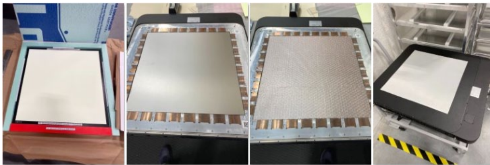
41 cm x 41 cm sensor DMI fabricated for Phoenix LLC for neutron radiography experiments. L-R: As received by Phoenix; coupled face down to a PerkinElmer 1621 flat-panel detector; compression cushioning added; flat panel cover attached.
