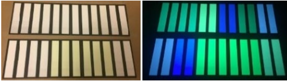
Control plates (under room and UV light) made by DMI for INL, on aluminum only, without a plastic substrate, used in conjunction with corresponding scintillator-coated wedged plastic slabs (described) to help determine the light output of each different scintillator and scintillator formulation alone, without the plastic substrate.
