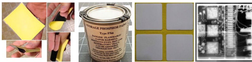
DMI flexible sensor (scintillator coating on aluminized Mylar); DMI storage phosphor paint; DMI ~ 8 cm x 8 cm cast sensors.
