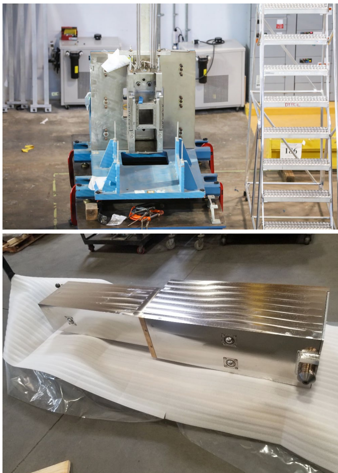
Core vessel (top) and shutter inserts (left) to be installed at VENUS during the SNS Winter outage, 2020/21.
