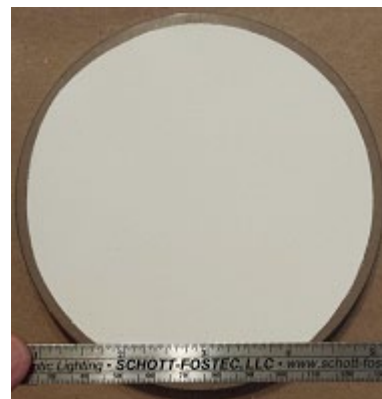
11 cm diameter, 1 cm thick, coherent fiberoptic plate coated by DMI with LSO:Ce scintillator (40-45 ns decay time to 1/e).
