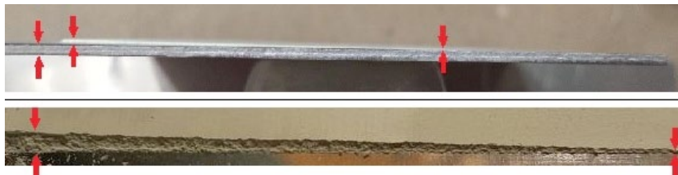
Cross sections of gradient sensor coatings on aluminum substrates.
