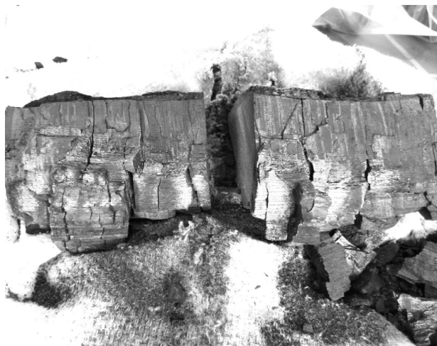
Fig. 2 Mock-up prepared from wood charred in a kiln for testing preservative measures.
