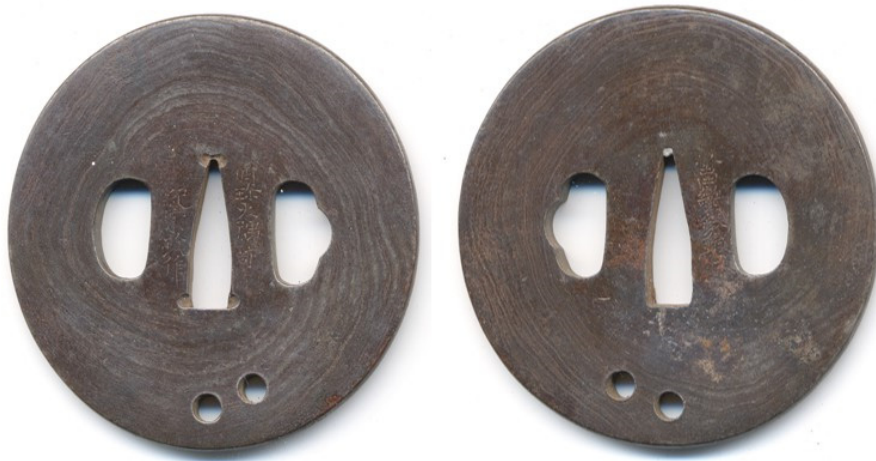
Fig. 1 Pictures of the two sides of the Myochin School tsuba analyzed using neutron laminography. Spiral lines running on the whole surface are visual evidence of the complex multilayered structure.
