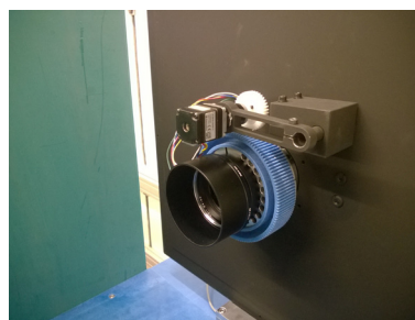
Photo of the autofocusing unit with the NIKKOR 85 mm lens (bellows were removed).
